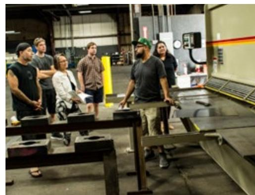
**JOSE LOPEZ**, in ballcap, a Standard Steel employee, explains how the company's new AccurShear metal shear works. It can slice half-inch steel plate.
