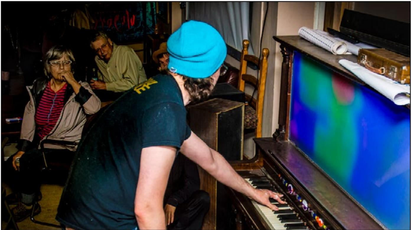
CYMASPACE founder and president Myles de Bastion demonstrates the LED piano he created in collaboration with Piano Push Play, a Portland-based piano-rescue group, and Lucid, a Portland design firm. The instrument's front panel was replaced with a grid of light-emitting diodes that respond to the sounds and tones of the piano. De Bastion
